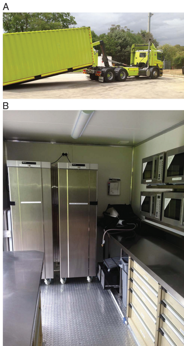
Fig. 5. Australian Capital Territory Fire and Rescue Platform on Demand (POD) welfare system deployed to long duration operational incidents. (A) External view, (B) internal view.
